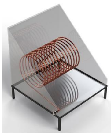
Figure (2) schematic diagram of the absorber room: dimensions, shape and copper pipeline conditions.
